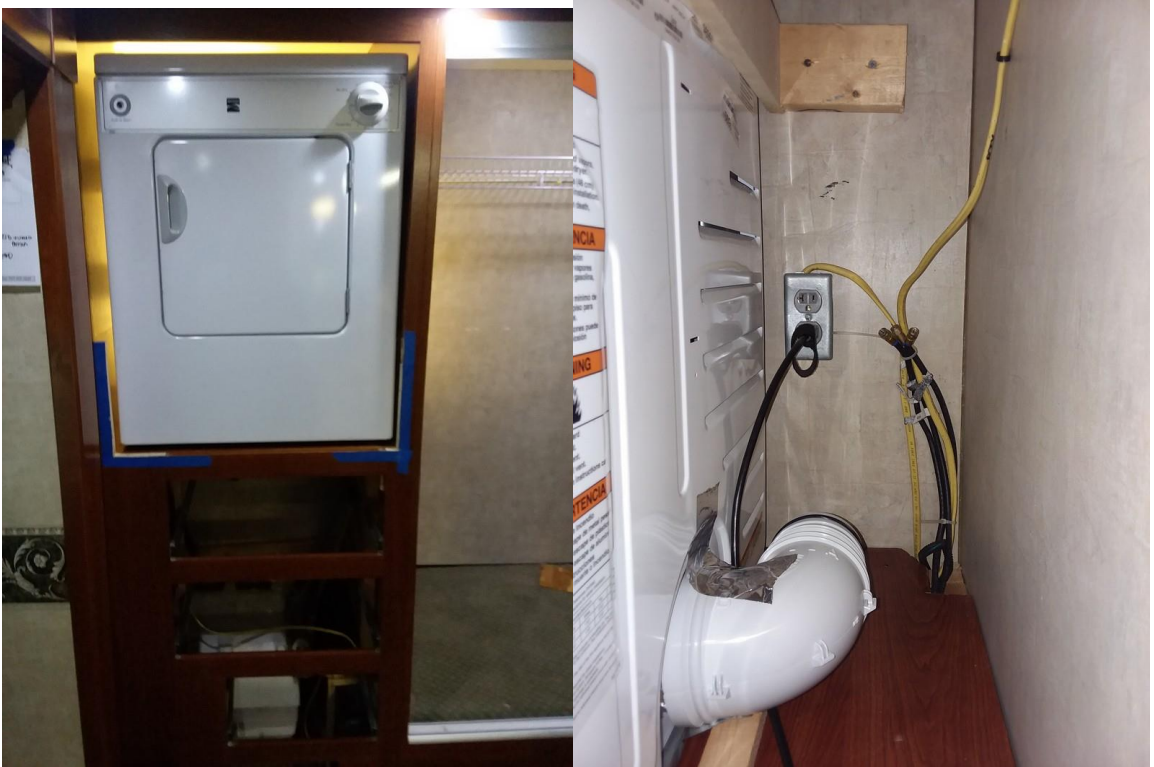
Jim and I easily picked the dryer up and put in place. I needed to perfectly locate where the hole for the dryer vent needs to be. I'll admit to being a bit nervous about drilling a 4" hole in my beautiful coach!!!!
