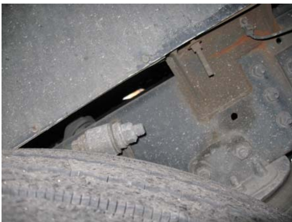
Crack in bracket aft of left rear tire
